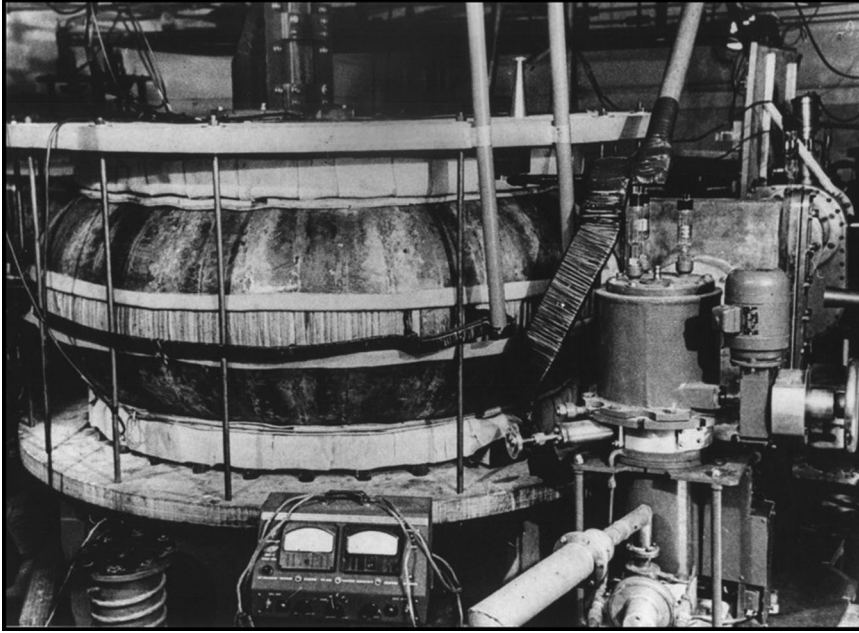
Figure 2. The world's first tokamak device: the Russian T-1. (Wikicommons.)
