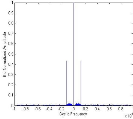
Fig. 1:  $|C_{42}^\alpha|$  of co-channel two QPSK overlapped signals.
