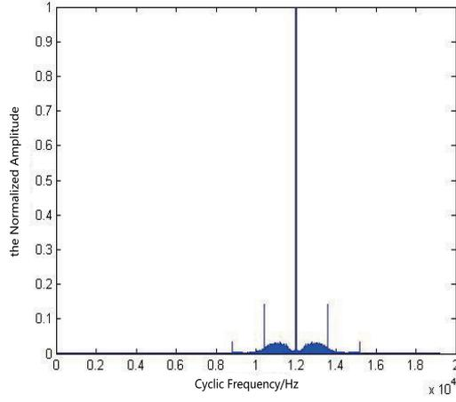
Fig. 3: The four-order cyclic cumulants  $|C_{40}^\alpha|$  of QPSK.
