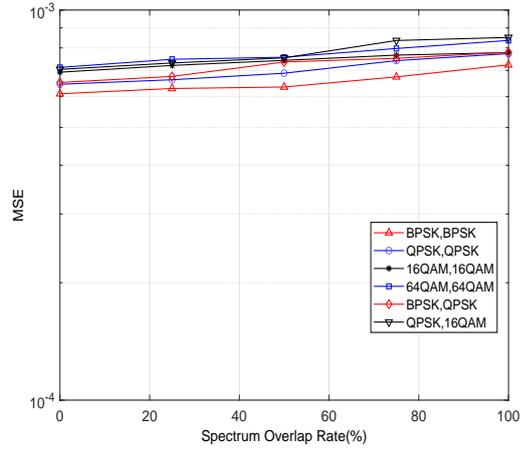
Fig. 12: Initial phase estimation performance of time-frequency overlapped signals with different spectrum overlapped rates.
