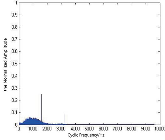
Fig. 4: The four-order cyclic cumulants  $|C_{42}^\alpha|$  of QPSK.
