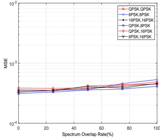
Fig. 7: Amplitude estimation performance of time-frequency overlapped signals with different spectrum overlapped rates.
