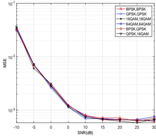
Fig. 10: Initial phrase estimation performance of time-frequency overlapped signals with different SNRs
