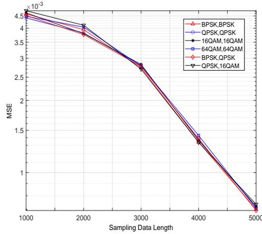
Fig. 11: Initial phase estimation performance of time-frequency overlapped signals with different data length
