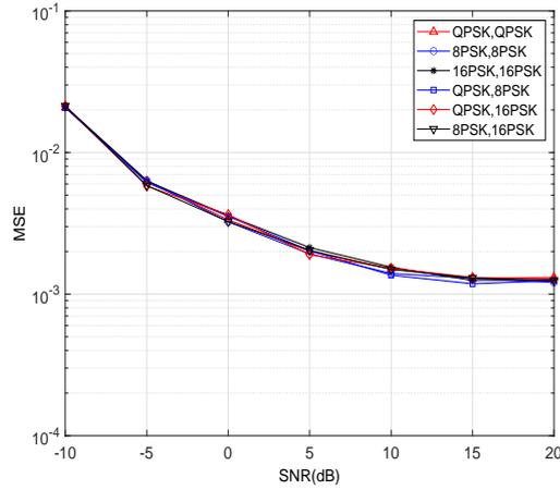
Fig. 8: Amplitude estimation performance of time-frequency overlapped signals when the power ratio is 1.2
