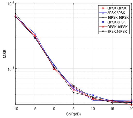
Fig. 5: Amplitude estimation performance of time-frequency overlapped signals with different SNRs.
