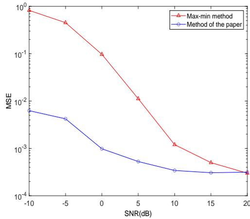
Fig. 9: Amplitude estimation performance comparison with different methods.
