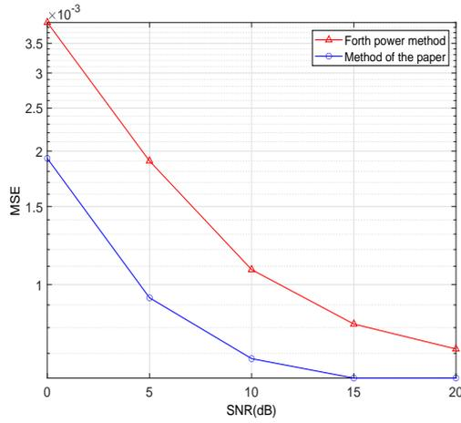
Fig. 13: Initial phase estimation performance comparison with different methods
