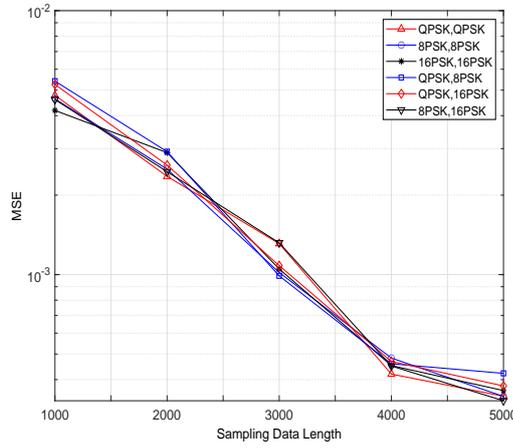
Fig. 6: Amplitude estimation performance of time-frequency overlapped signals with different data length.
