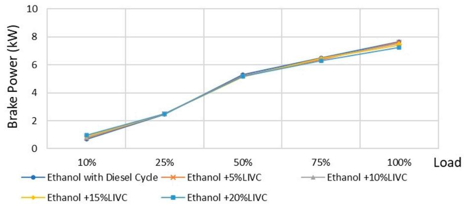
Figure 19. BP(kW) of ethanol engine with LIVC Miller Cycle.
