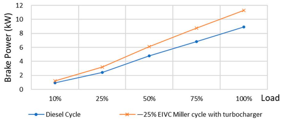
Figure 11. Comparison of BP between diesel engine and EIVC Miller cycle turbocharger diesel engine.
