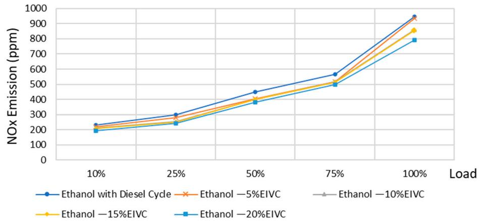
Figure 18. NOx emission(ppm) of ethanol engine with EIVC Miller Cycle.
