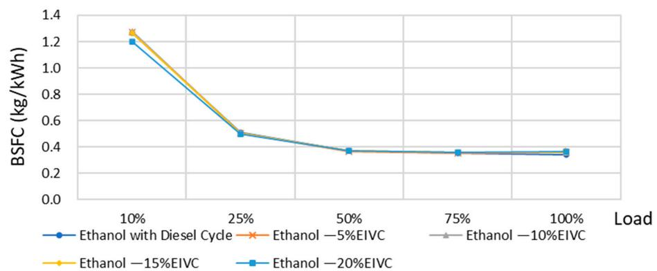
Figure 16. BSFC(g/kWh) of ethanol engine with EIVC Miller Cycle.
