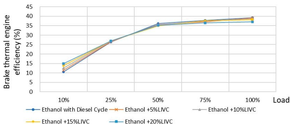
Figure 21. BTEE(%) of ethanol engine with LIVC Miller Cycle.
