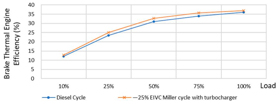
Figure 12. Comparison of BTEE between diesel engine and EIVC Miller cycle turbocharger diesel engine.
