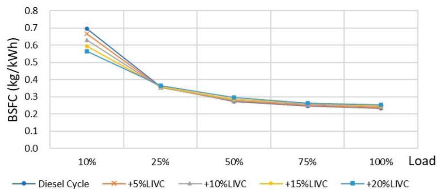
Figure 9. Comparison of BSFC under diesel engine LIVC Miller cycle.
