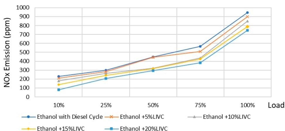
Figure 22. NOx emission(ppm) of ethanol engine with LIVC Miller Cycle.
