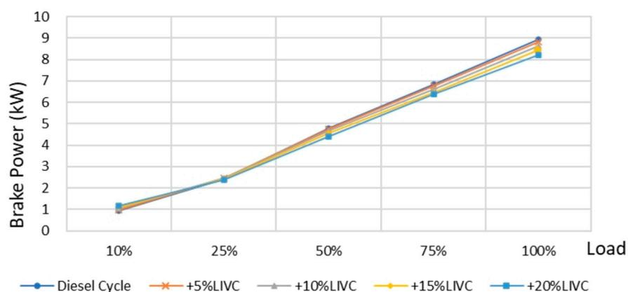
Figure 7. Comparison of BP under diesel engine LIVC Miller cycle.
