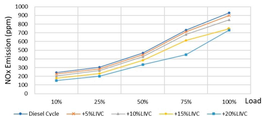
Figure 10. Comparison of NOx emission under diesel engine LIVC Miller cycle.
