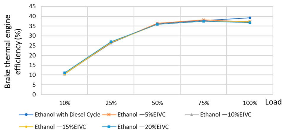
Figure 17. BTEE(%) of ethanol engine with EIVC Miller Cycle.
