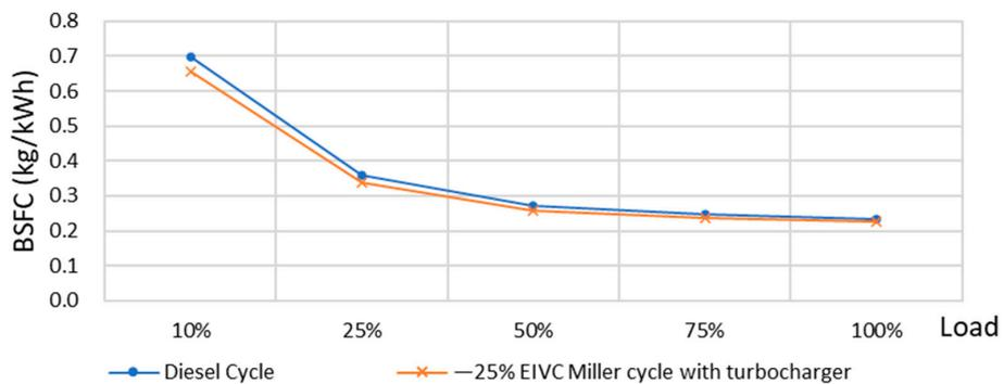
Figure 13. Comparison of BSFC between diesel engine and EIVC Miller cycle turbocharger diesel engine.
