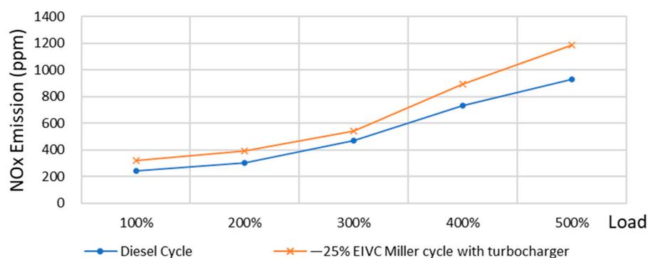
**Figure 14.** Comparison of NOx between diesel engine and EIVC Miller cycle turbocharger diesel engine.
