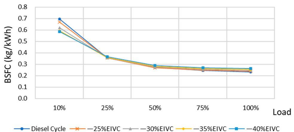
Figure 5. Comparison of BSFC under diesel engine EIVC Miller cycle.
