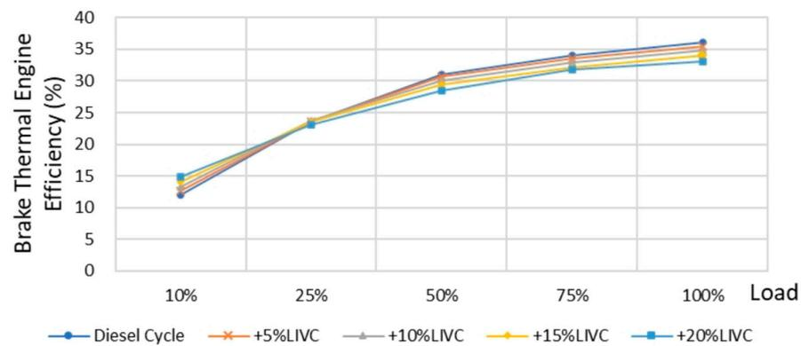
Figure 8. Comparison of BTEE under diesel engine LIVC Miller cycle.
