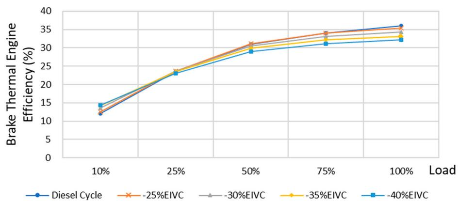
Figure 4. Comparison of BTEE under diesel engine EIVC Miller cycle.
