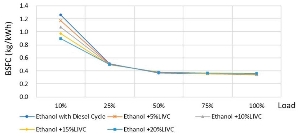
Figure 20. BSFC(g/kWh) of ethanol engine with LIVC Miller Cycle.
