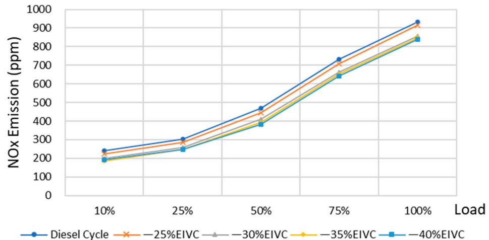
Figure 6. Comparison of NO<sub>x</sub> emission under diesel engine EIVC Miller cycle.
