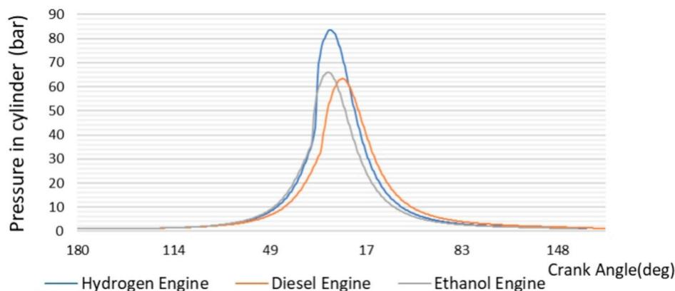
**Figure 23.** Diesel, ethanol and hydrogen engine in-cylinder pressure.
