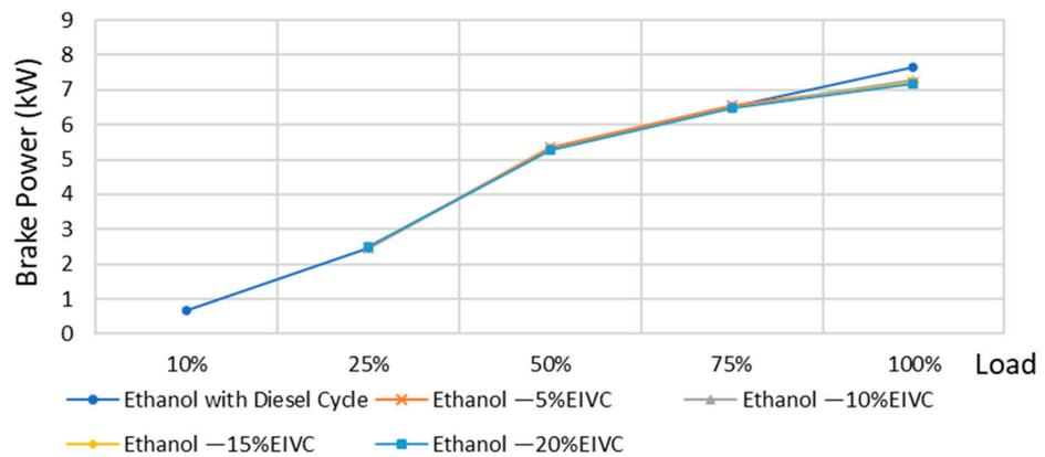
Figure 15. BP(kW) of ethanol engine with EIVC Miller Cycle.
