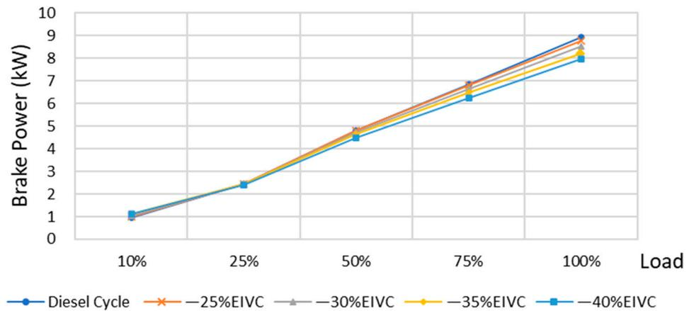
Figure 3. Comparison of BP under diesel engine EIVC Miller cycle.
