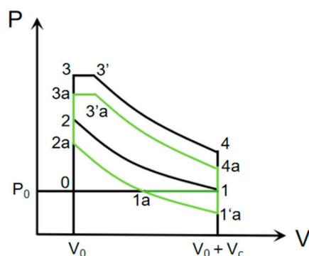
Figure 1. Dual cycle [5] and Miller cycle (EIVC) [6].
