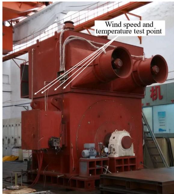
Fig. 10. Prototype experimental platform.
