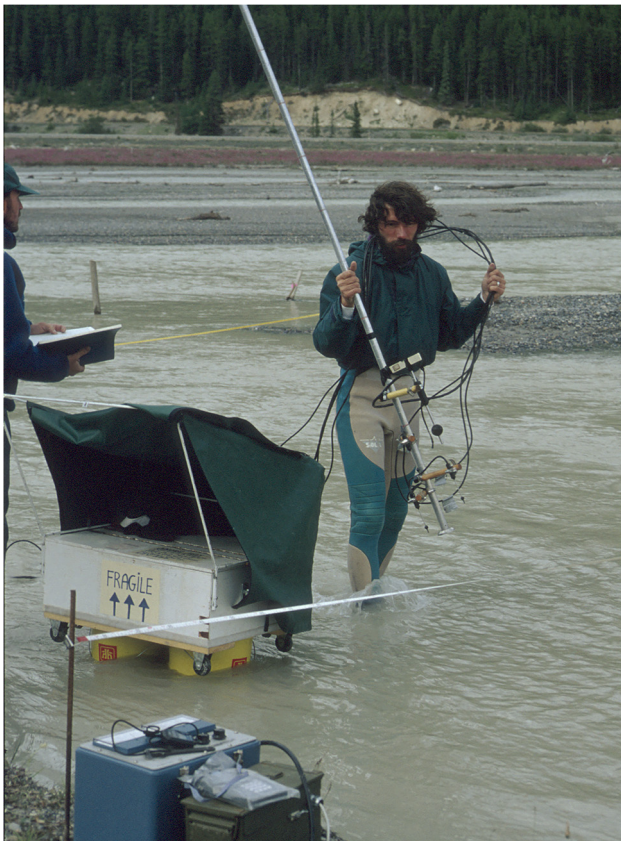
Fig. 1. New technology for flow measurement. André Roy measuring flow structure in a braid confluence using electromagnetic current meters. Photograph: R.I. Ferguson.
