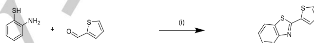
Scheme 2. Synthesis procedure for the reference compound BTaz-Th : (i) sodium metabisulfite, DMF, reflux, 2 h.
