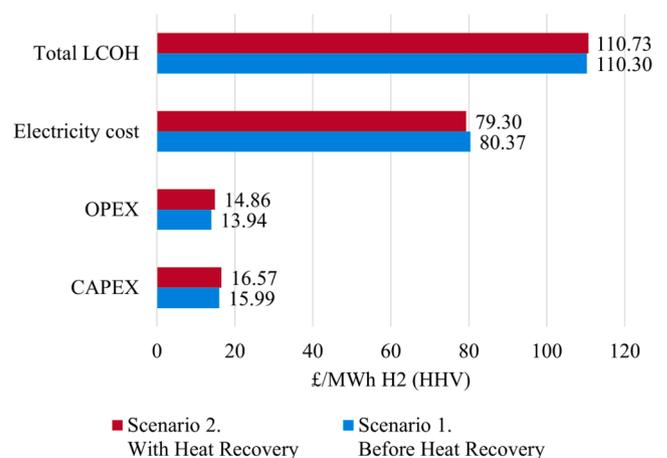
**Fig. 11.** Levelised Cost Estimates (£/MWh H<sub>2</sub> (HHV)) for 10 MW PEM Electrolysis System using offshore wind electricity.
