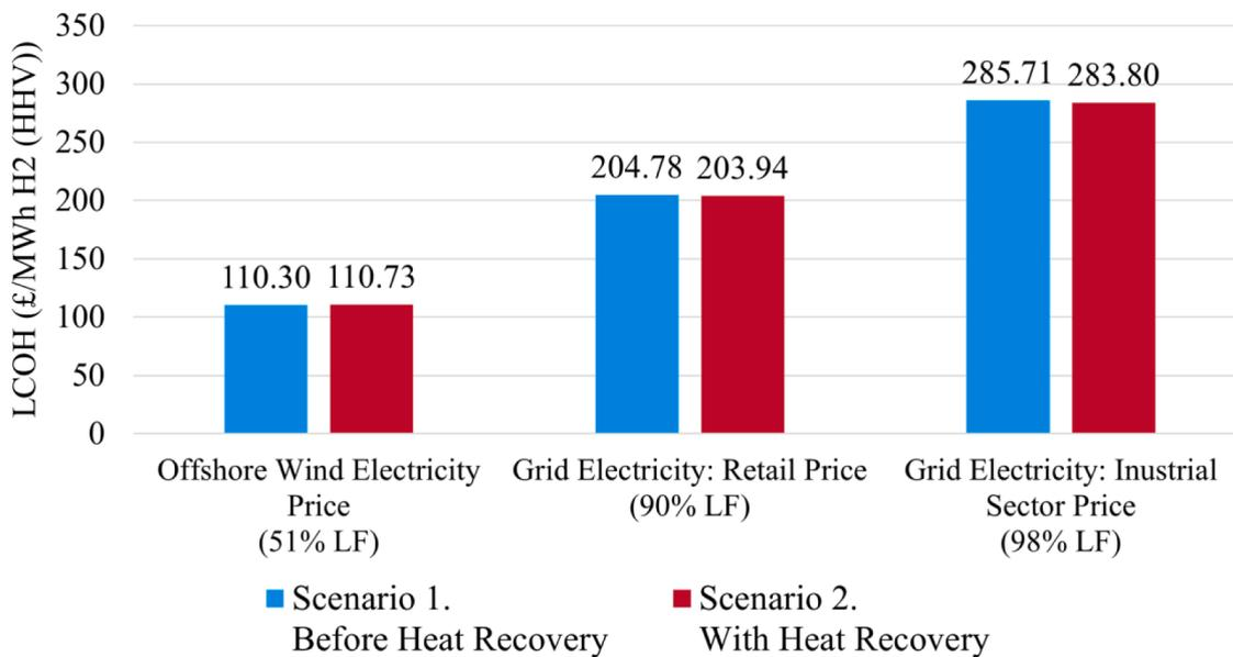
Fig. 13. Comparison of LCOH with different electricity sources.
