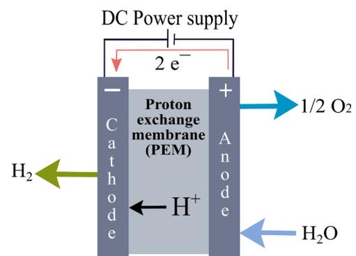
Fig. 1. Schematic of a PEM electrolyser cell.
