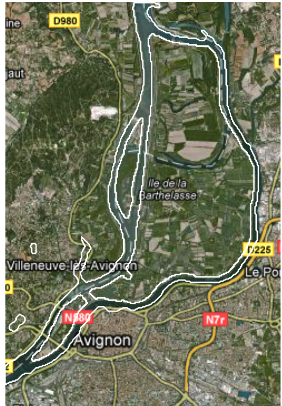
Figure 4: River network segmentation from a colour image using the new algorithm. Flow conservation is satisfied at junctions, illustrated by a significant change of width, and along branches, as illustrated by a slow change of width. (©2010 Google - Imagery ©2010 TerraMetrics, Map data ©2010 Tele Atlas.)
