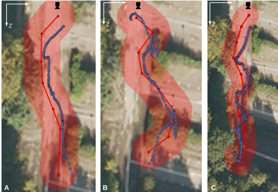
Figure 7. Three exemplar tracks (A,B,C) plotted on geo-referenced satellite imagery (blue) with corresponding ground truth obtained from hand-held GPS tracking units (red with  $\pm 5m$  error boundary plotted).
