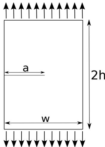
Figure 1: : Edge crack plate under a uniform load.
