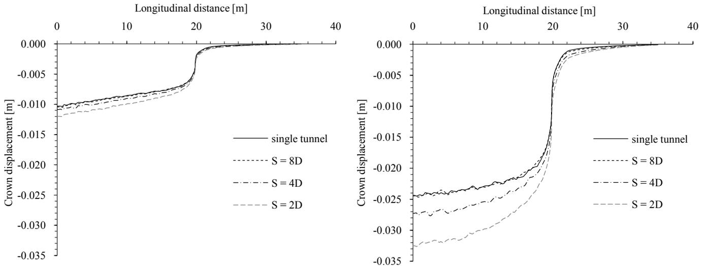
Figure 4: Crown displacement profiles along the opening length: (a) at end of excavation; (b) approximately 40 days after excavation.
