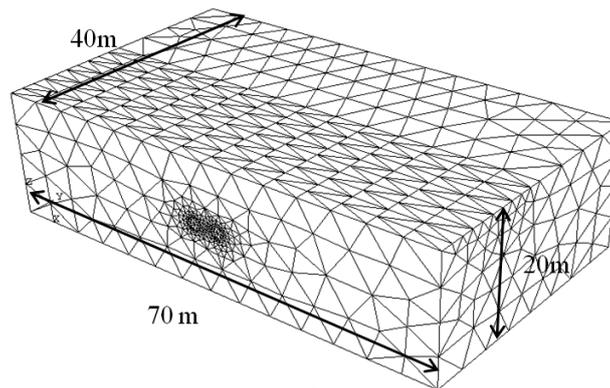
Figure 3: Three-dimensional FE mesh ( $S=2D$ ). 38465 elements, 53023 nodes.
