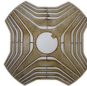
Fig.13. Rotor lamination.
