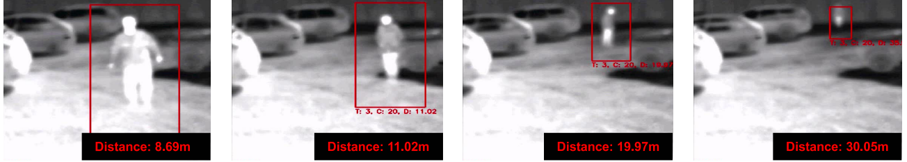
Figure 2. Photogrammetry facilitates the approximate recovery of a camera to target distance for an example target (person) without any need for additional (active) range sensing [5]
