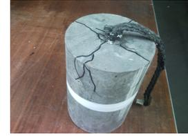
Figure 4: Sample 5TR - Showing rupture of fibre and cracking of concrete
