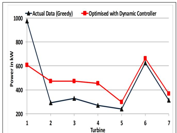
Fig 3: Power optimised with dynamic farm controller wind speed 8ms/ ± 0.5 and parallel to turbine array
