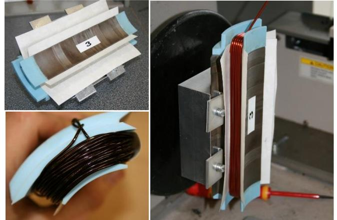
Figure 2: A stator segment of a FSCW synchronous reluctance machine. Top left: Unwound segment with end caps and insulation. Bottom left: Wound segment. Right: Bobbin winding.
