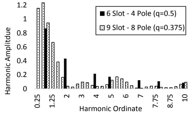
Figure 4: MMF harmonic spectrum of a fractional slot concentrated windings with  $q=0.5$  and  $q=0.375$ .
