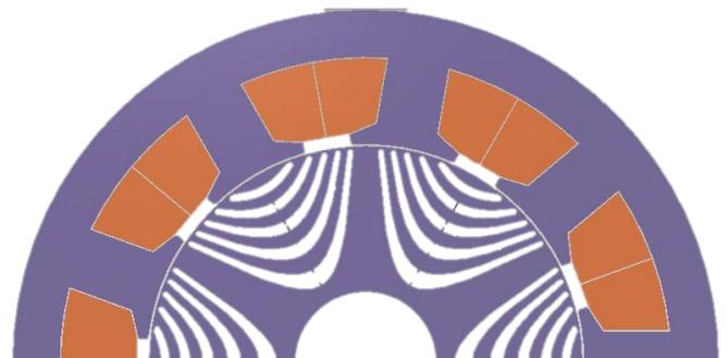
Figure 5: The designed 9 slot 6 pole machine used in the study.
