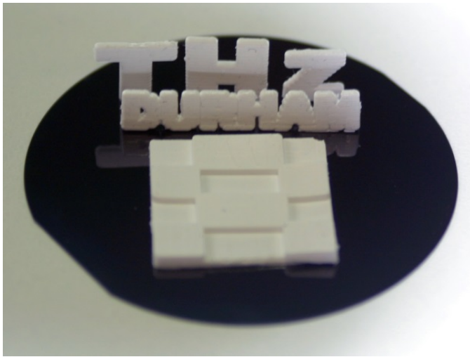
Fig. 2. Phase shift mask generated from a Hadamard matrix of order 16, for coded aperture imaging in the THz region. \epsilon_r = 2.5 throughout.
