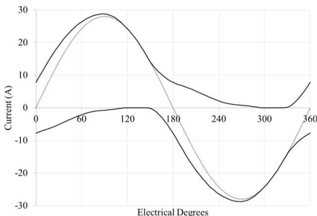
Fig. 12: FE simulated current plots for the six phase symmetric 'dot-dot' configuration driven from a three phase bridge, showing a single sinusoidal current source (dotted line), and the resultant 180 degree separated phase currents (solid line)
