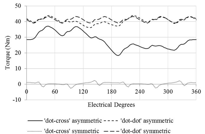
Fig. 8: FE simulated torque output for different winding configurations driven from a three phase bridge under sinusoidal current control
