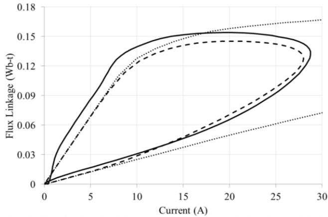
Fig. 9: FE simulated  $\psi$ - $i$  characteristics for a single phase with the symmetric 'dot-dot' winding configuration, showing static characteristics in the unaligned and aligned positions (dotted lines), a single phase dynamic loop (dashed line), and a dynamic loop arising from full six phase operation (solid line)
