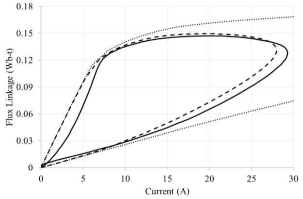
Fig. 10: FE simulated  $\psi$ - $i$  characteristics for a single phase with the asymmetric 'dot-cross' winding configuration, showing static characteristics in the unaligned and aligned positions (dotted lines), a single phase dynamic loop (dashed line), and a dynamic loop arising from full six phase operation (solid line)
