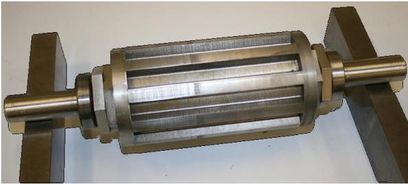
Fig. 3: Rotor from the six phase prototype SRM
