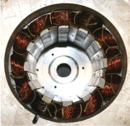
Fig. 2: Constructed six phase prototype SRM
