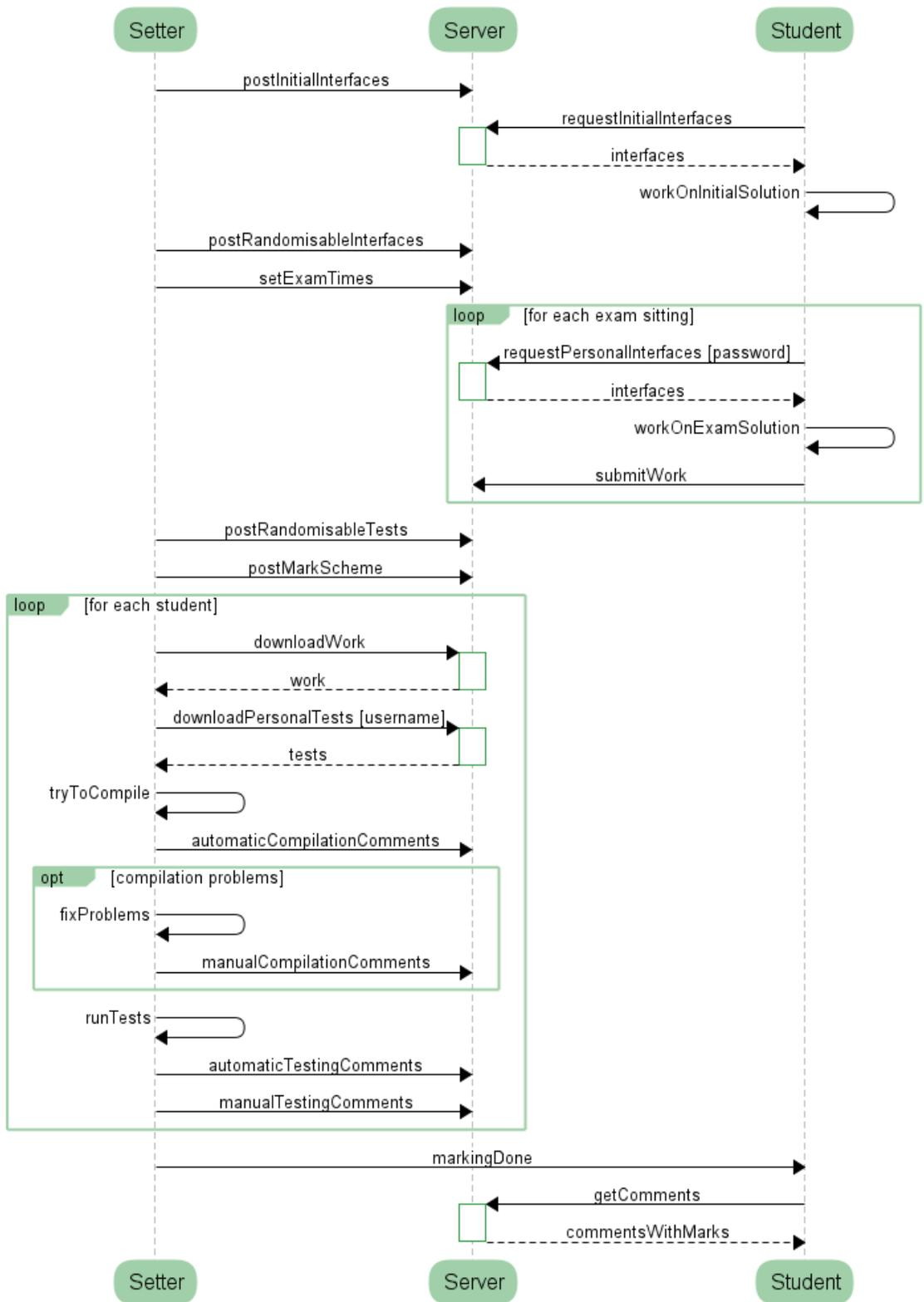
Figure 1: Sequence diagram for setting and marking process with blending and randomisation
