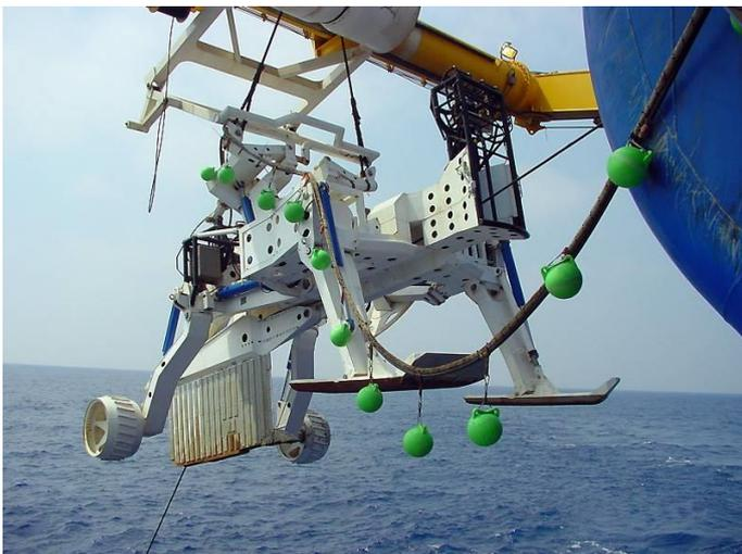
Figure 1. Seabed cable plough (Courtesy of Serge Delestaing).
