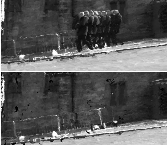
**Fig. 6.** Top: A slow moving pedestrian with approximately 50% self-overlap between frames. Bottom: Successfully removed from mapping solution.
