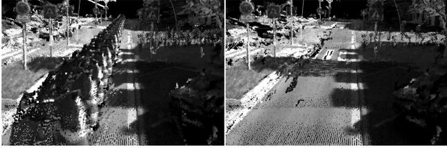
**Fig. 2.** Left: A car driving forwards, ahead of the logging platform, reconstructed multiple times cluttering up the global point cloud. Right: Moving object removed from the final reconstruction.
