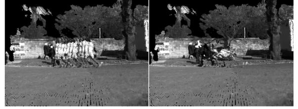
**Fig. 3.** Left: Moving object reconstructed multiple times. Right: Moving object masked out of the reconstruction process.
