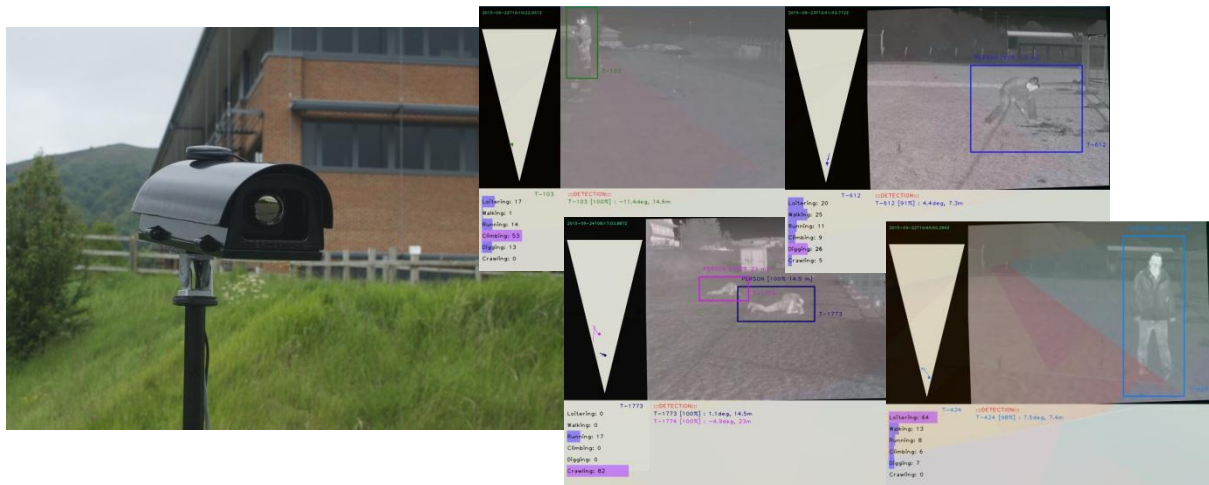
Figure 3: Durham University developed ASM (photograph left) based on a Thermoteknix MIRICLE 307K thermal camera. The screenshots on the right hand side show behaviour classifications as follows (clockwise from top left): Climbing, Digging, Loitering, Crawling. Each screenshot comprises the thermal image (top right pane) with detection box overlay, the geolocation and tracking window (top left pane) and the classification histogram (bottom pane).
