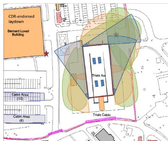
Figure 11: The sensor laydown implemented for the SAPIENT demonstration. Showing two PTZ ASMs (Red Stars), three Thermal Imager ASMs (blue cones), four radars with steerable beams (green lobes), one 30m laser scanner and three 20m laser scanners (orange segments). Also shown is the Herras fencing (solid brown line) surrounding an inner protected area containing four shipping containers (dark blue rectangles).
