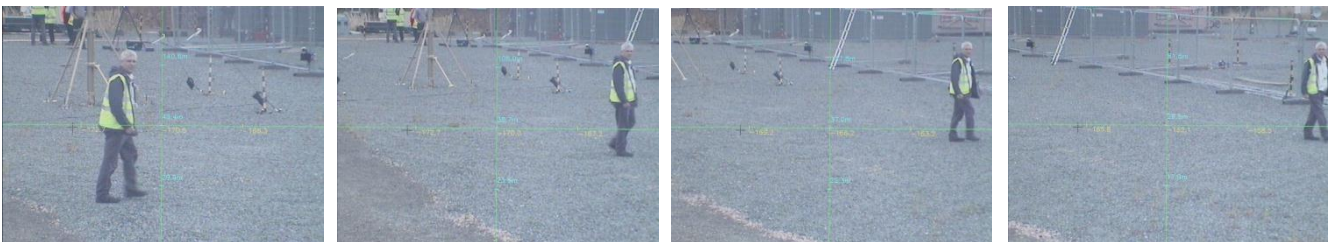
Figure 7: several successive screen shots from the QinetiQ PTZ ASM showing "follow mode". Note the background features which indicate how the ASM has autonomously changed its field of view to keep the target in the frame.
