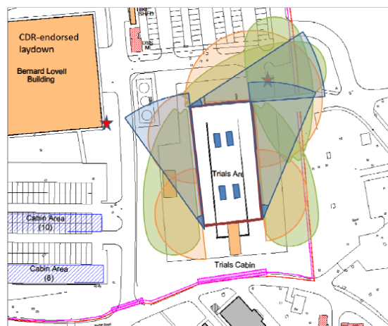
Figure 11: The sensor laydown implemented for the SAPIENT demonstration. Showing two PTZ ASMs (Red Stars), three Thermal Imager ASMs (blue cones), four radars with steerable beams (green lobes), one 30m laser scanner and three 20m laser scanners (orange segments). Also shown is the Herras fencing (solid brown line) surrounding an inner protected area containing four shipping containers (dark blue rectangles).
