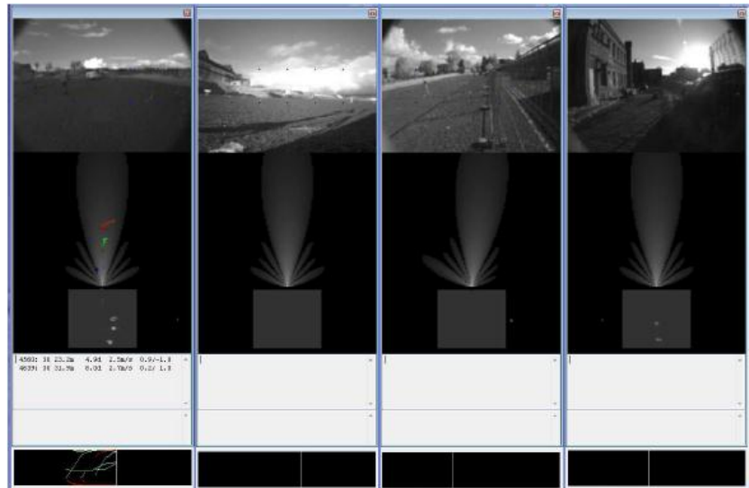
Figure 13: Radar ASM engineering GUI showing: a black and white video image of the scene; a “radar cone” display showing the radar beam, and detected plots & tracks, a range-Doppler map (objects further up the map being further away, objects moving towards the radar appear to the left of centre and objects moving away from the radar appear to the right), a list of current tracks and a plot of the classification over a moving time window
