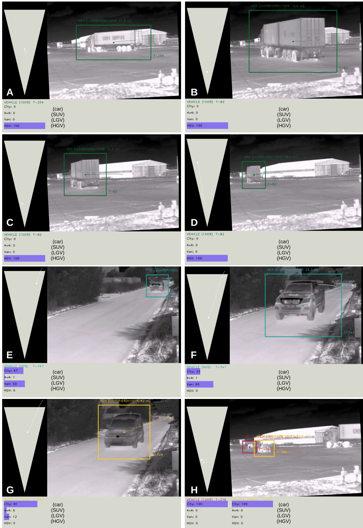
Figure 4. Examples of real-time vehicle detection, type classification and tracking in infra-red imagery with associated geo-referenced 3D track (based on using HOG features with SVM classification).
