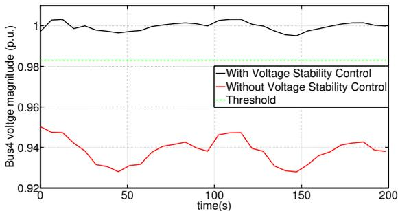
(c) Bus 4 voltage magnitude with v.s. without voltage control.
