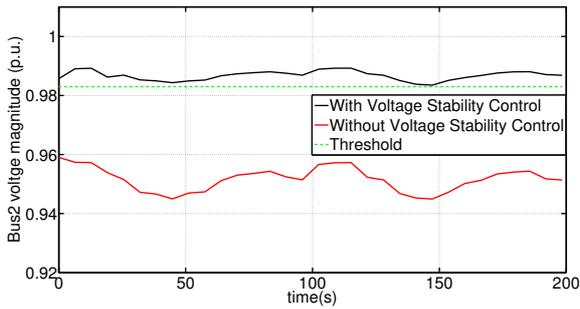
(a) Bus 2 voltage magnitude with v.s. without voltage control.
