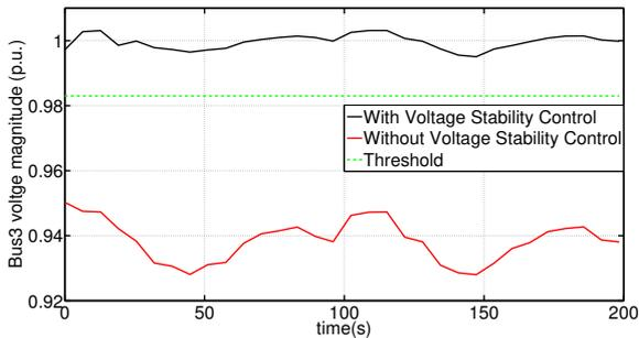
(b) Bus 3 voltage magnitude with v.s. without voltage control.
