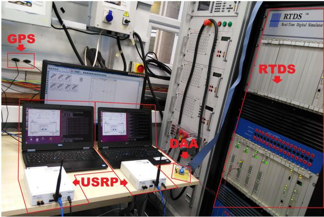
Fig. 1. The implemented prototype of Smart Grid testbed running 4 bus power system test case with USRP, RTDS and Data Acquisition and Actuator (DAA) module.
