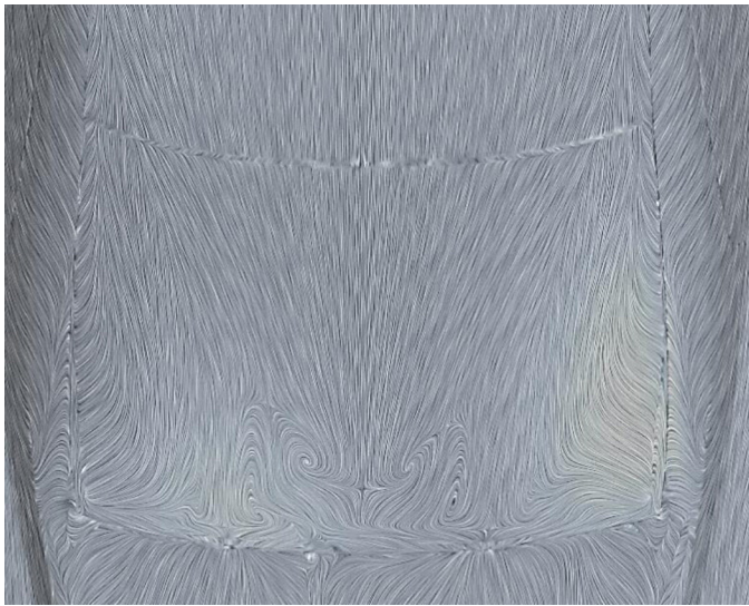
Figure 9. Limiting streamline pattern calculated in CFD for 30% Volvo S60 without the overhead strut
