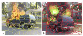
**Fig. 4**. Exemplar superpixel based fire region localization (A) and subsequent CNN based classification (B).
