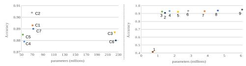
Fig. 3. Fire detection performance for variations of the AlexNet architecture (left) and InceptionV1 architecture (right).
