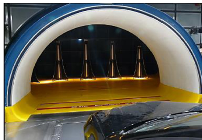
Figure 3. Pininfarina wind tunnel turbulence generation system [14].
