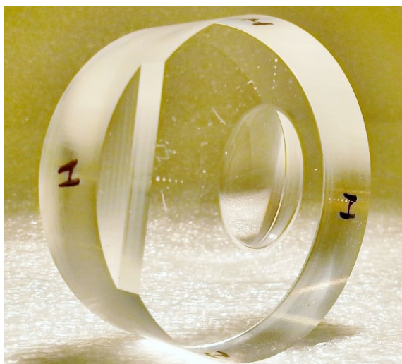
(a) Photo of the plasma mirror. The surface is registered from the front plane, the flat at the edge, and the outer diameter.
