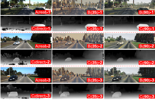
Figure 6: Results demonstrating the importance of style transfer. Left column shows results with no domain adaptation. Middle column contains results with [35] as domain transfer and the right column indicates results with [90].
