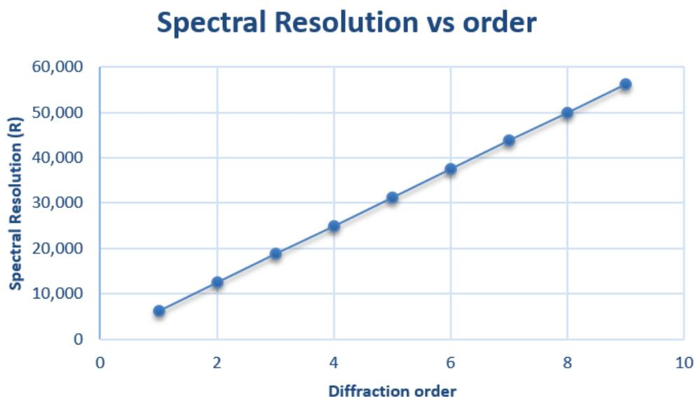
Figure 4. Linear dependence of the spectral resolution with the diffraction order for a groove density of 250 lines/mm and a pupil diameter of 25 mm.
