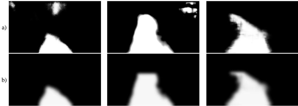
Fig. 5 Example output path confidence maps, a) before and b) after post processing
