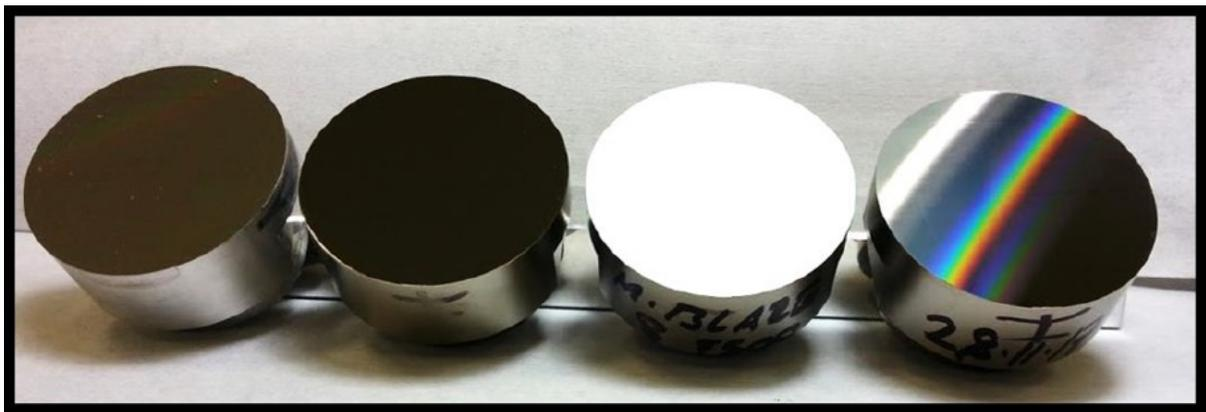
Figure 3: 4 freeform diffraction gratings machined according to the specification in Table 1.
