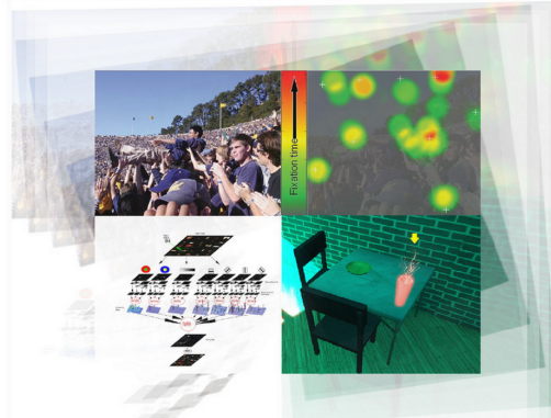
Figure 1: Top: Subtle Gaze direction, input image for modulation (left). Gaze distribution for modulated image (right). White crosses indicate locations preselected by researchers for modulation [Bailey, McNamara et al. 2009]. Bottom Left: Schematic of the iLab Neuromorphic Vision, a comprehensive set of C++ classes for the development of neuromorphic models of vision [Baldi and Itti 2010]. Bottom Right: In a Search task, a High Level Saliency predictor highlights a vase at a consistent with the context location signifying an easy recovery [Koulieris et al. 2013].
