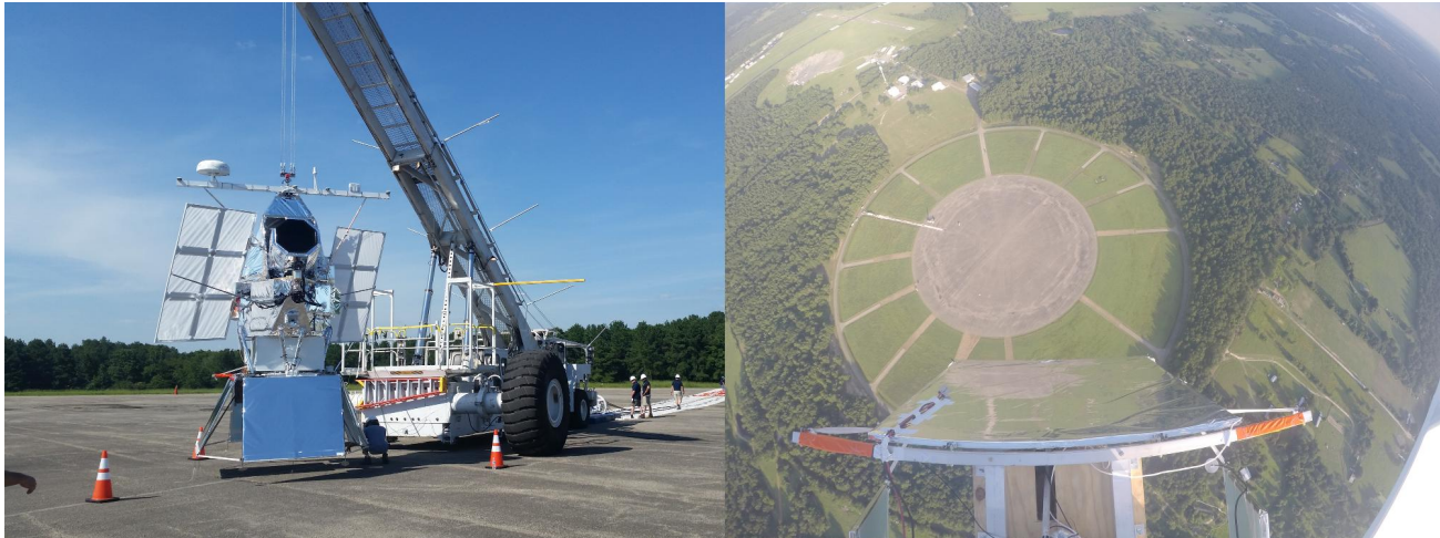
Figure 5. The SUPERBIT 2016 Palestine campaign and flight; (left) the SUPERBIT gondola on the launch pad hours before launch on June 30, 2016; communications antennas and mass-model solar panels were used to accurately emulate SPB configuration; (right) footage taken from a downward facing GoPro camera on the SUPERBIT gondola seconds after launch from the CSBF launch pad
