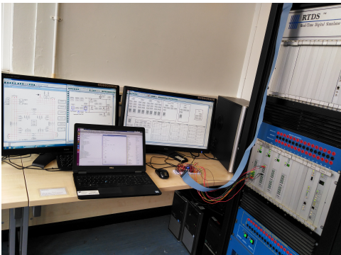
Fig. 4. The real-time estimation setup with RTDS, Matlab and DAA module.
