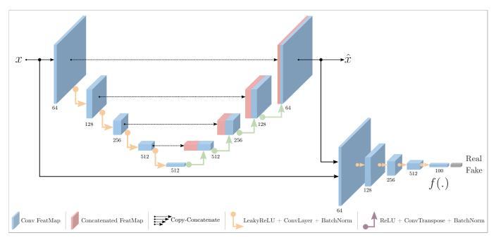
Fig. 3: Details of the proposed network architecture.
