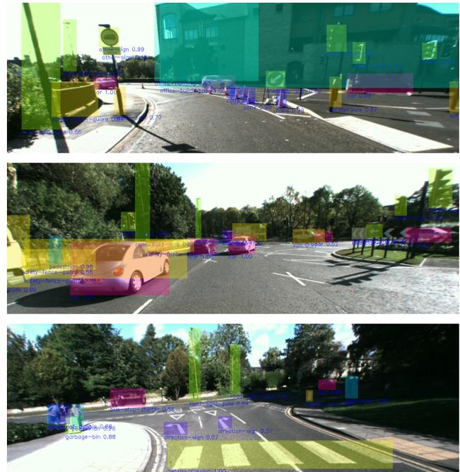
Fig. 1. Exemplar extended real-time multiple class object detection with attribute estimation within an urban environment.
