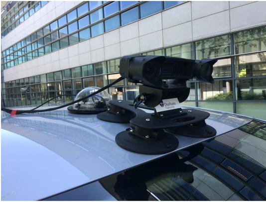
Fig. 3. The vehicle equipped with stereo camera and combined GPS/IMU system
