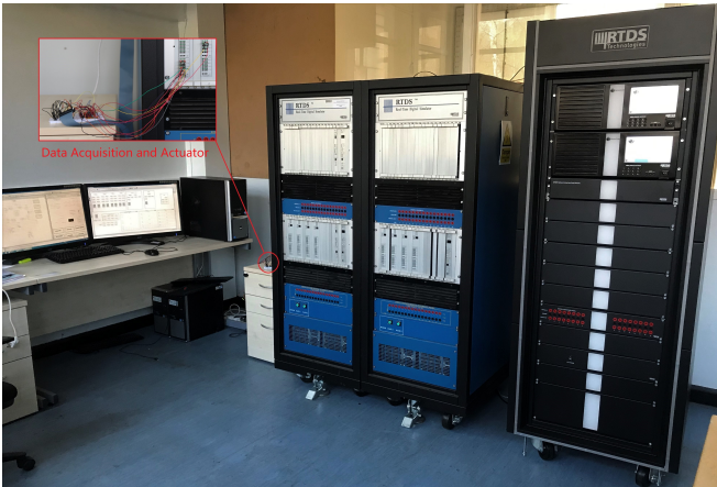
Fig. 4. Interactions Setup of Matlab/PC, RTDS and DAA.
