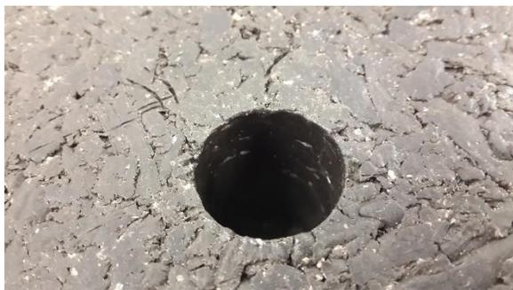
Figure 4. Augered pile hole (diameter 20 mm)
