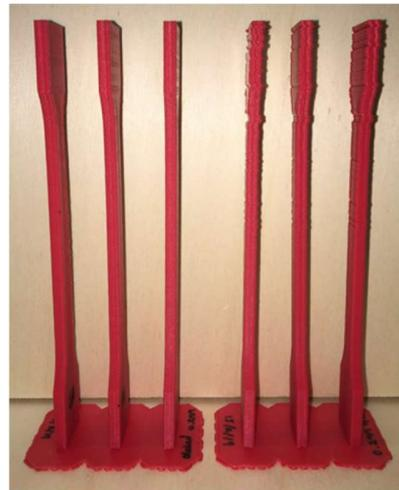
Figure 9: Closed enclosure (left) compared to open enclosure printing (right). Rafts located at the print bases
