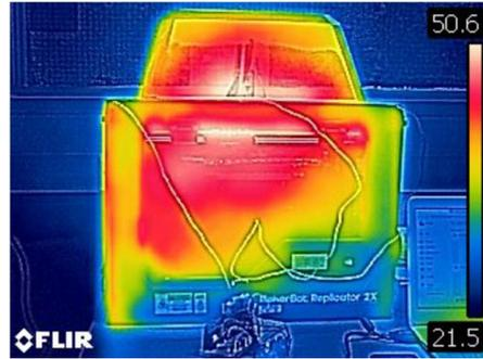
Figure 16: Thermal image of heat distribution at the start of a print
