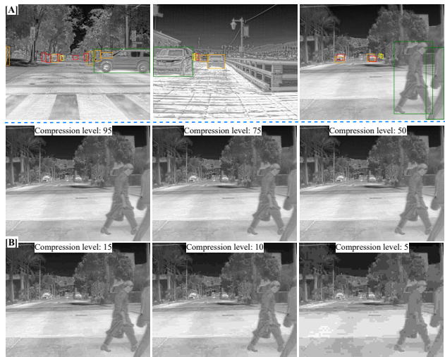
Figure 1. Exemplar infrared imagery from FLIR [16] containing different classes with varying object areas in bounding boxes: tiny, small, medium, large [A]. Example imagery at different lossy compression levels [B].
