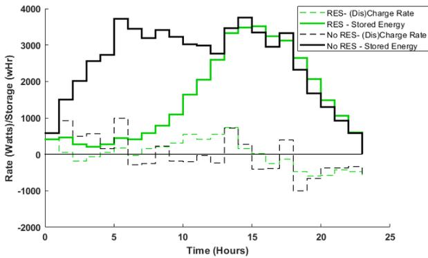
Fig. 4. Battery storage levels of Case 3 in Scenarios 1 and 3.
