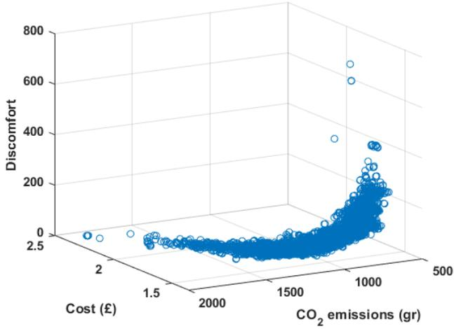
Fig. 1. Pareto Frontier evaluating cost, CO<sub>2</sub> emissions and discomfort, obtained after evaluating the MOIA.
