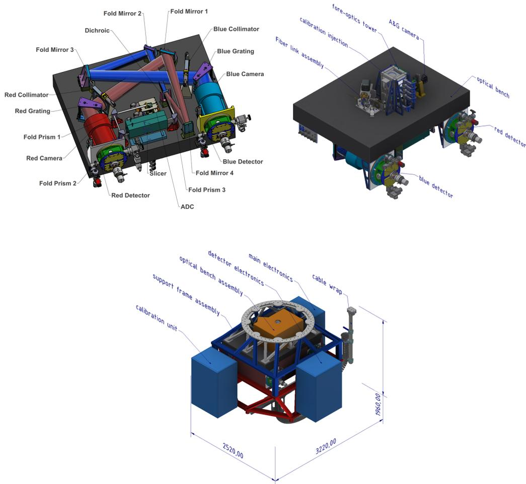
**Fig. 4.** Mechanical concept for CUBES: The general layout of the main mechanical components is shown. For reference, the Telescope Adapter has a diameter of about 1.5 m. The Fore-Optics Assembly is located near the center of the bench, while the spectrograph opto-mechanics are ‘hanging’ on the bottom side of the same bench.
