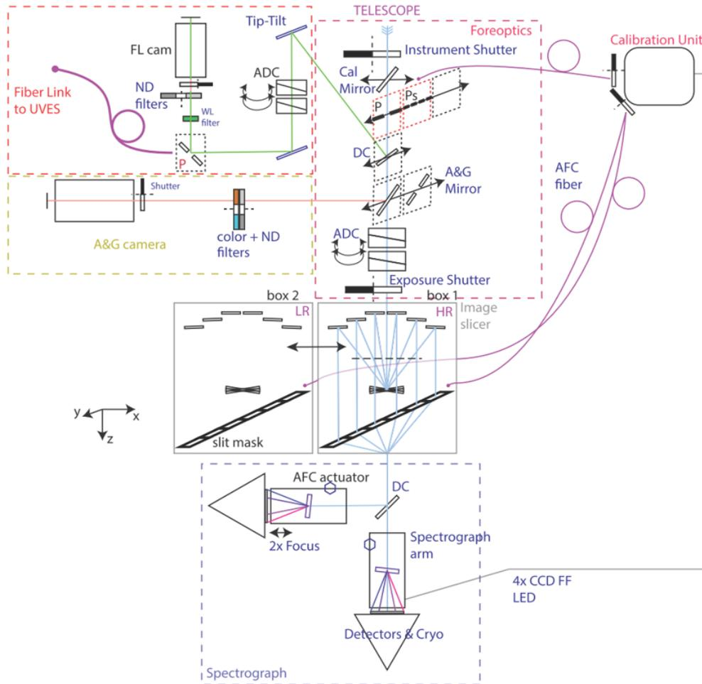
**Fig. 3.** Functional design of CUBES. Light path is from the top to the bottom. The shown acronyms are: FL cam (fibre-link A&G camera), ND filters (Neutral Density filters), WL filter (Wavelength filter), ADC (Atmospheric Dispersion Corrector), P (single Pin-hole mask), Ps (multi pin-holes mask), A&G (Acquisition and Guiding), Cal mirror (Calibration mirror), DC (Dichroic), AFC (Active Flexure Compensation), LR (Low Resolution), HR (High Resolution), Cryo (Cryocooler), FF LED (Flat-Field LED).
