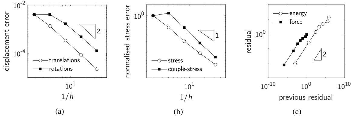
Figure 1: Convergence with mesh refinement of (a) translations/rotations and (b) Cauchy stress/couple-stress. Newton-Raphson convergence through a single loadstep is depicted in (c).
