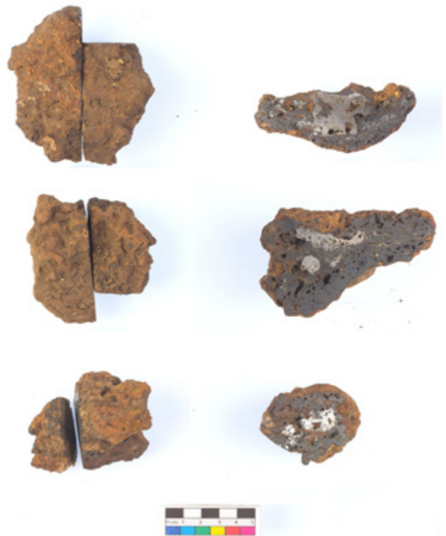
Figure 9.3. Photographs of top view and section of three metallic-iron rich slag cakes from Bagendon. The topmost example was not sampled, while the middle is analytical sample IoA-BAG-S-3, and the bottommost is sample IoA-BAG-S-4.
