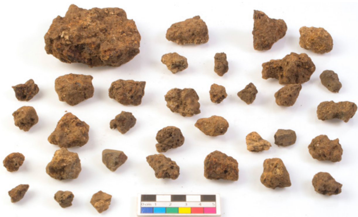
Figure 9.1. Photograph of typical slag assemblage from Bagendon (context 80-40). The top left slag is a slag cake, while the others are amorphous.
